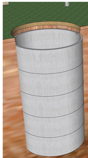
3. Sink Other Caissons
