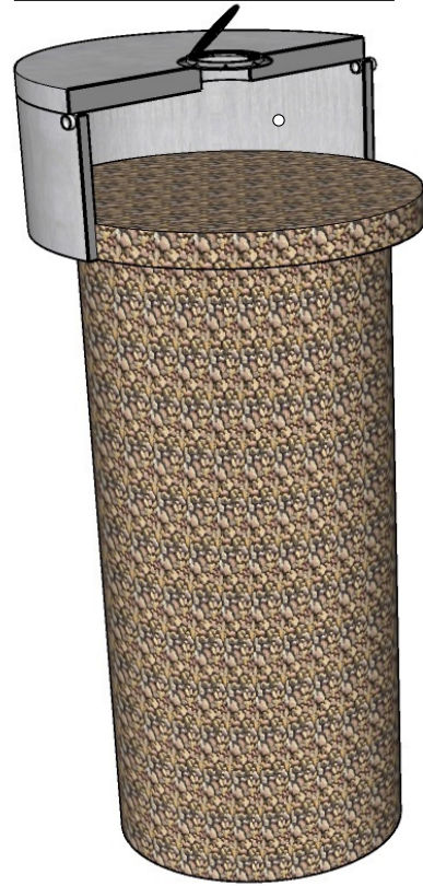
A. ONE-CAISSON WELL 20' SHAFT
